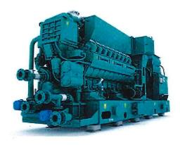
Alternator – Several alternator sizes offer selectable voltage and temperature rise with low reactance 2/3 pitch windings; low waveform distortion with non-linear loads, fault clearing short-circuit capability, class F or H insulation (see Alternator Data Sheet for details), bearing and stator RTDs and anti-condensation heater. Mechanically strengthened for use on utility paralleling with unreliable grid.
