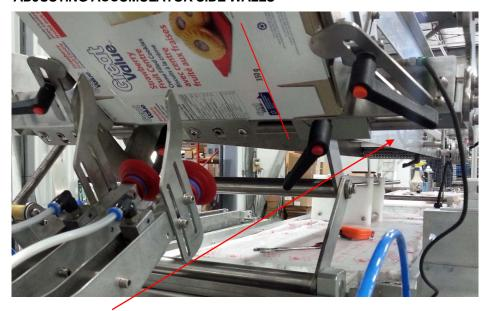
Belt Conveyor Wall is factory aligned with the front edge of the lug conveyor and when changing over to new carton the folding on the right side of the carton has to be aligned with the edge of the belt conveyor wall. Than the side wall of the accumulator has to be adjusted to the flap size. Next step is to adjust the left accumulator wall to new carton size.
