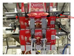
Release the ratchet clamps on both sides of the accumulator output carton holders. Move holders mounts up or down to adjust it to new carton's length. You can slide the links horizontally as well to adjust horizontal holders position. Carton holders are to hold cartons in the gravity portion of the accumulator. While adjusting the holders position make sure that pick up head pulls a single carton out from the accumulator.
