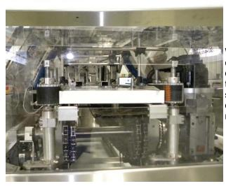
With the conveyor set wider than the depth of the carton insert the manually erected carton into the orange discharge belts. Rotate the adjuster screw in the direction of conveyor flow to close down conveyor sides until the side flaps are flat but the carton is not deformed. It is easiest to do this with the screw at the near the discharge of the machine.
