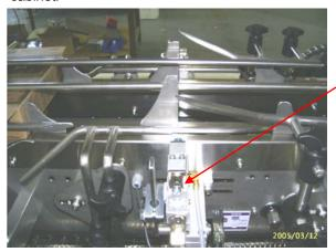
Jog the machine until the pushing lug edge is against the glue gun nozzle.
