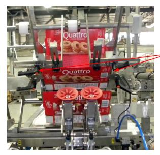
Loosen ratchet clamps to adjust side holders. Sam approach as for top carton holders: make sure vacuum feeder pulls out a single carton without disturbing other cartons.
