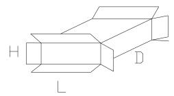
Box Length, Height and Depth are defined as shown. The dimension commonly referred to as Height may be called Width in this Manual when more obvious.
