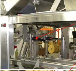
There are 2 sets of ratchet clamps to adjust top rail (guide) horizontally and vertically to new carton height/depth.
