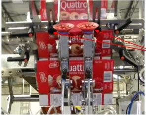
To adjust the holders vertically loosen both nobs and slide them to new position. When adjusting (positioning) the holders make sure the pile of cartons in the gravity portion does not sag (bend) in the middle.
