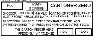
This screen is where the main timing value for the cartoner is set. The machine must be jogged until the carton is about to leave the glue area. Pressing **SET** button will enter the value of the encoder at that moment into the setting for machine zero. This becomes the basis for all of the timing of the glue guns, the carton vacuum release and the position to stop the machine when running in **INDEXING** mode.
