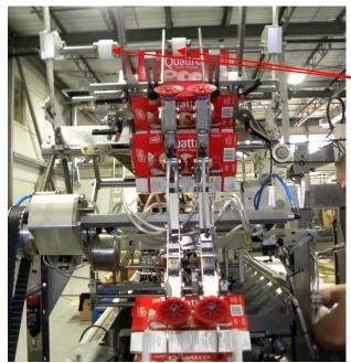
The adjustable roller is to control the number of cartons that is transferred from motorized portion of the accumulator to gravity portion of the accumulator.
