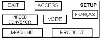
This screen is the path to all of the other screens. Touch the button for the desired screen. **EXIT** button returns the display to the previous screen. Machine is available only in **SERVICE** level access.
