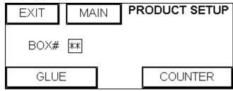
This screen has the buttons to go to **GLUE** and **COUNTER** settings. The BOX # setting is to choose next carton # for which **GLUE** settings have been already preset and **COUNTER** screen will show production data for this carton # as well.
