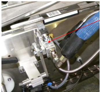
Release the glue gun clamp and adjust the gun height for desired glue line position on the box.
