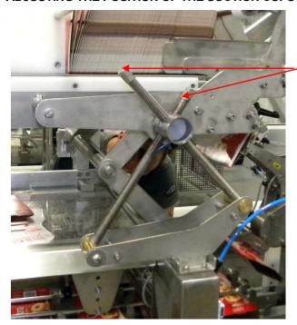
Adjust the height of the accumulator with the adjuster screw at the side of the accumulator to bring the center of the suction cups to 1.5 inches above the fold.
