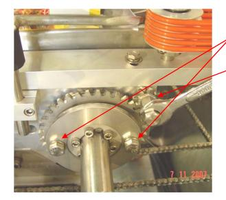
Release two locking screws on the lug chain driving sprocket.
