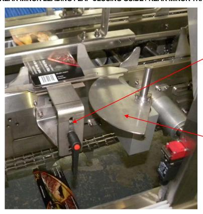
This guide is to close rear minor leading flap. It is adjusted vertically (ratchet clamp) and horizontally (2 screws)
