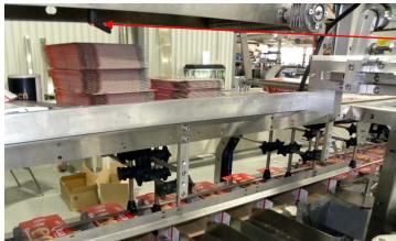
To move the left wall release this ratchet clamp and move the wall to adjust it to new carton depth. Tighten the clamp when done.
