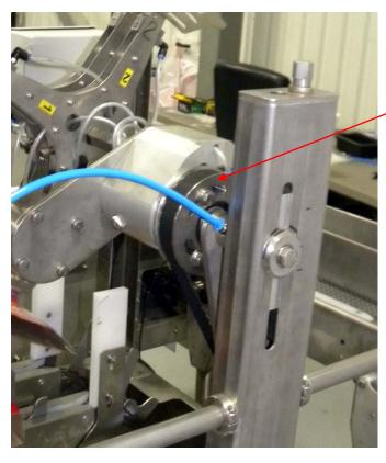
Loosen the bolts that lock the head drive. The rotary head should move by hand. Holding the rotary head in the vertical position, jog the conveyor until the trailing edge lugs (pushers) are 1.5 inches from the center of the suction cups. Lock the head drive clutch.
