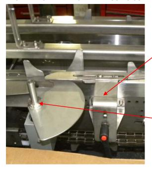
This guide is to close front minor leading flap. It is adjusted vertically (ratchet clamp) and horizontally (2 screws).
