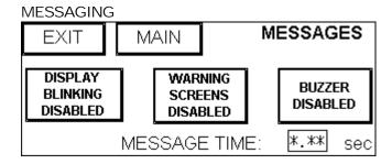
This is the screen to set the posting time for messages in the status window of the main screen and it gives the option for warning messages/display blinking or not. It has also the button to disable sound alarm.
