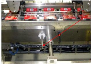
If the conveyor is narrower than the depth of the carton, rotate the adjustment hex-head screw against direction of conveyor flow to widen the conveyor.
