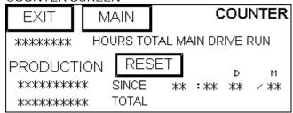
This screen has the button to reset the production counter and it shows date and time of the production period.
