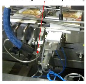
If the gun activates- the pneumatic valve solenoid is out of order. If the gun does not activate- the gun is clogged or the gun spring is overtensioned. See **GLUE GUN SPRING ADJUSTMENT.**
