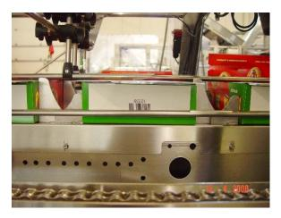
Allow visible clearance between carton and lugs, in order to prevent box deformation and marking.
