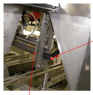
2. Turn the ratchet to move the prebreak module up or down to adjust it to new carton/new feeder position
