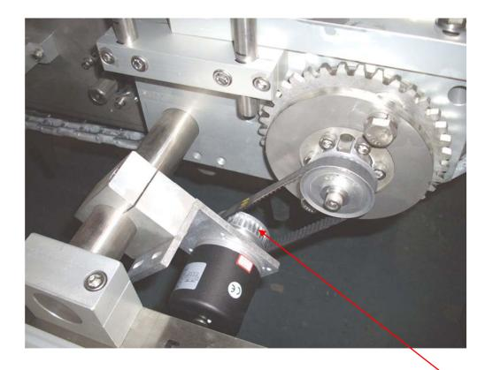
Do not spray water flow directly on machine's and printer's encoder. (if installed)
