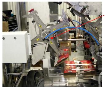
Jog the Cartoner until the rotary head has suction cups aligned **vertically** over a pocket in the main chain.
