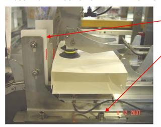
Adjust the bumpers to about half of the length of the sides (Height) of the carton so that the carton will open and fall into the pocket in the chain
