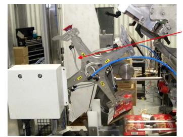
Jog until the rotary head suction cups touch the carton in the accumulator.
