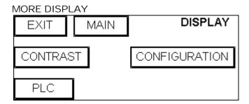
This screen is to adjust display contrast and to go to PLC settings screen. CLOCK button opens clock screen.
