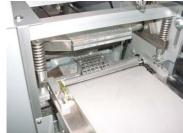
Dual roll holder with automatic splicing unit
