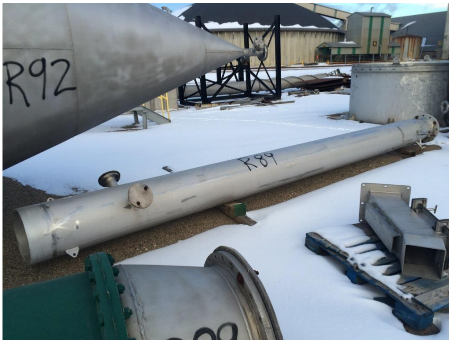
Figure 4. Photograph of the large diameter pipe connection the crystallizer body to the recirculation pump.
