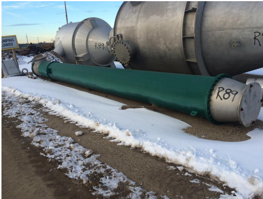
Figure 3. Photograph of shell and tube heat exchanger.
