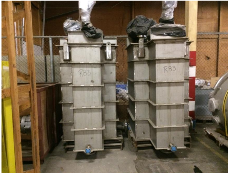
Figure 1. Photograph of the two fully assembled flocculation mix tanks
