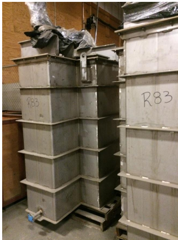
Figure 2. Photograph of the two fully assembled flocculation mix tanks
